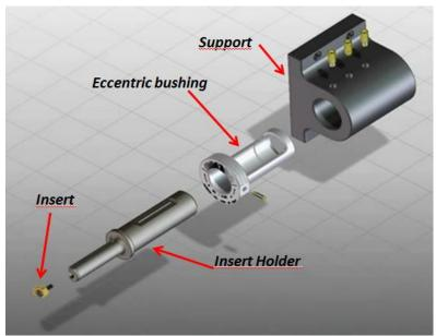
Picture No.1- Composition of a REV BROACHING TOOL system
