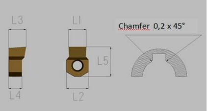
**Picture No.7 –** *Standard insert for the production of keyways*
