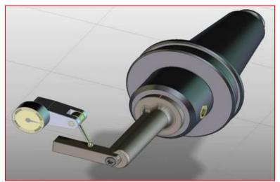
Picture No. 2- Illustration of the tool alignment system
