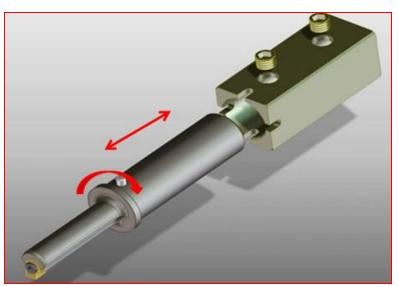
Picture No. 3- A simple application to rotate the position of the insert by 90 degrees
