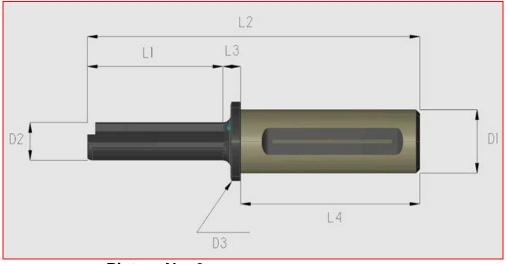
Picture No. 6 – Standard insert-holder spindle
