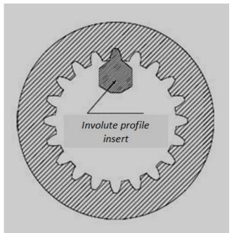
Picture No.8 – Production of an internal gear with M=2 ; Z=20 ; AP=20°
