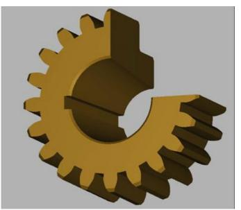
Picture No. 8- Broaching of keyway on a tampered bore.
