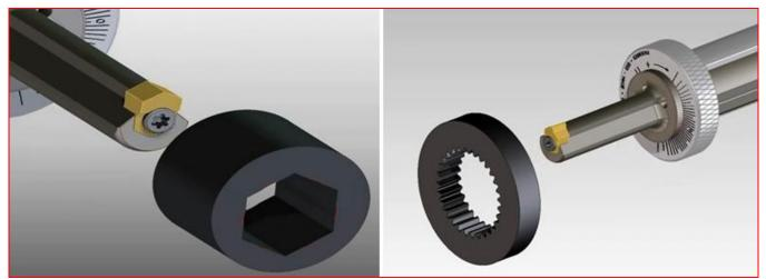
**Picture No. 5** – In addition to keyways, several other profiles can be obtained
